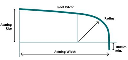
Note: Metroll takes no responsibility for variances on sheets curved from drawings. A template should be supplied to ensure accuracy. The minimum recommended curving radius is 450mm.
