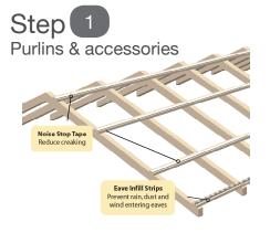
1. Ensure that your roof pitch is at least 5°, ie. 88mm rise per lineal metre. This will ensure adequate water run off.
