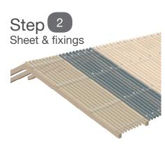
1. Ensure that the UV surface protected side faces the sun. This is the side of the label and the inkjet marking. When installed as a wall or fence it is recommended that the UV protected side is facing the most sun. The life of the sheet may be shortened and discolouration may occur due to the unprotected side being exposed to UV radiation. 2. The sheet can be easily cut with a pair of shears, a fine-toothed handsaw or a circular saw with a cut-off blade suitable for plastic.
