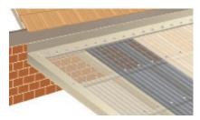
AGAINST A WALL/FASCIA - Fit metal barge capping to edge of sheet and metal apron flashing at the wall or fascia.
